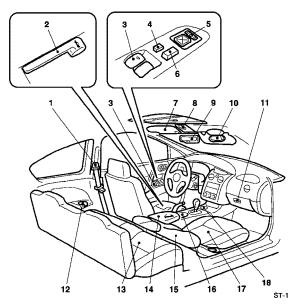
1. Seat belt  $\rightarrow$  p. 68 Adjustable seat belt shoulder anchor (for front seats)  $\rightarrow$  p. 73
